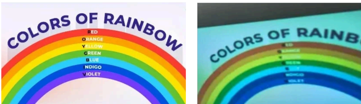
Figure 24: 640x480p at 20 fps: test image (left), frame from IMX219 (right)
